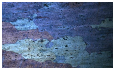
Fig. 2 Aluminum 7075 (20X) with almost any precipitation
